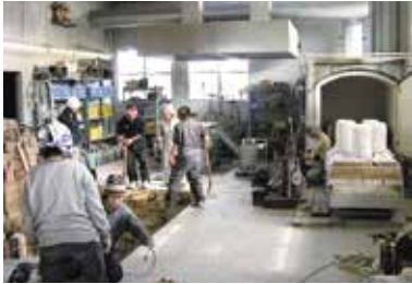
Metal Casting and Molding Workshop A workshop dedicated to “metal casting,” which consists of creating forms by pouring melted metal into a plaster pattern. Fully equipped with a tilting furnace that can contain up to 100 kg, a gas kiln, a hoist crane, etc.
