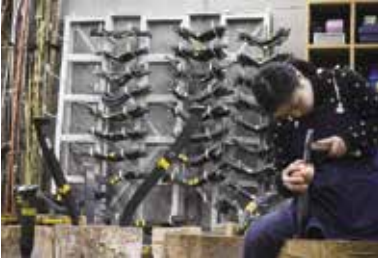
Hammering and Embossing Workshop A workshop dedicated to “hammering,” which consists of molding metal by striking and extending it. Fully equipped with more than 80 types of dolly blocks, a gas burner for thermal processing, etc.
